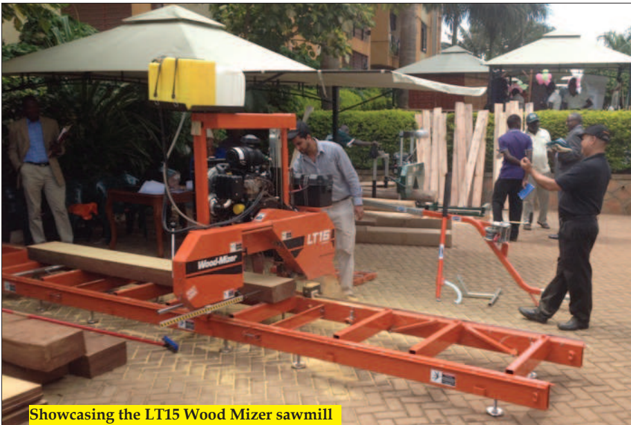
A processor showing the operation of a portable woodland sawmill
